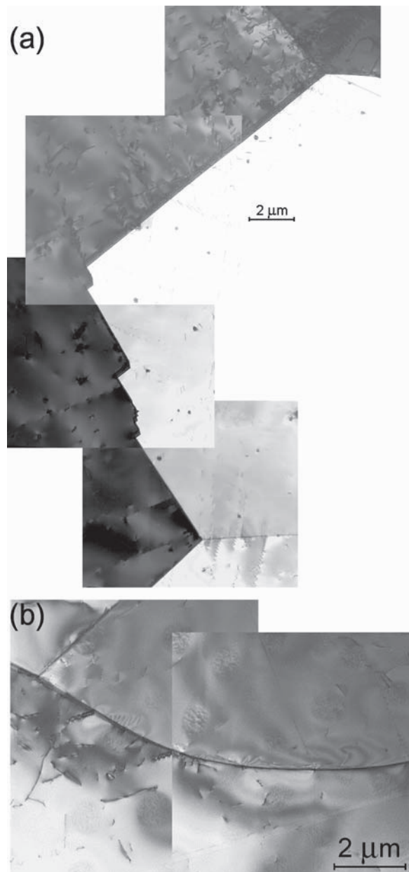
Figure 10 TEM micrographs of grain boundaries in 316L stainless steel heat-treated (a) at 1100°C for 1 h and (b) at 1300°C for 15 min [108].
